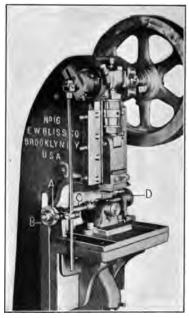
Fig. 1. Press with Attachment for Perforating Shell shown in Fig. 3
